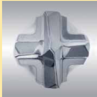
Thanks to optimum 4 x 90° symmetry, all four carbide cutting edges function evenly and do not seize up on hitting reinforcing steel
