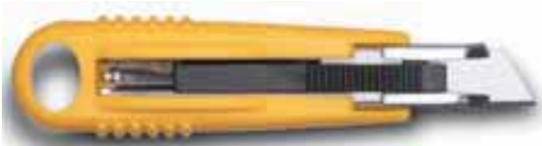
For left handed knife simply remove blade and rotate 180° and reassemble
