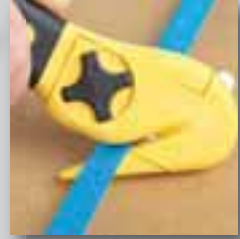
Cut strapping at 45°
