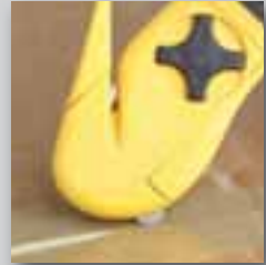
Tape slitter on the back of Tusk
